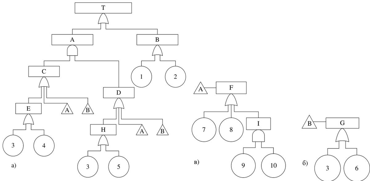
**Figure 3. Fault tree of a fire detection and alarm system for qualitative analysis.**
