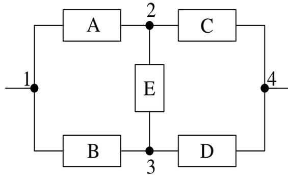
**Figure 1. Bridge structure reliability network.**
